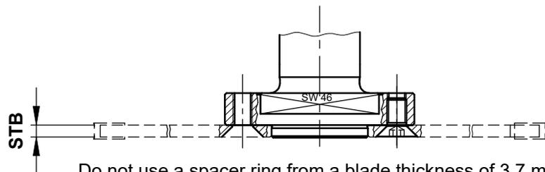
Do not use a spacer ring from a blade thickness of 3.7 mm
